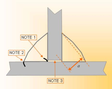
Dominant fatigue cracks in partial penetration welds
